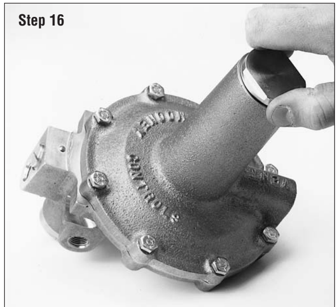
Figure 37 - Screw the Cover with O-Ring into place.
