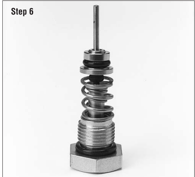
Figure 29 - Stack the Return Spring, Stem Guide, Orifice Spring, Plug and Stem, Orifice, Orifice O-Ring, and Back-up Washer on the Closing Cap.
