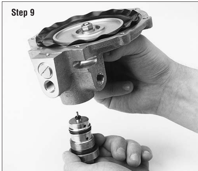
Figure 31 - Insert Body Insert (Cartridge) with lubricated Stem O-Ring into the Pilot Body.
