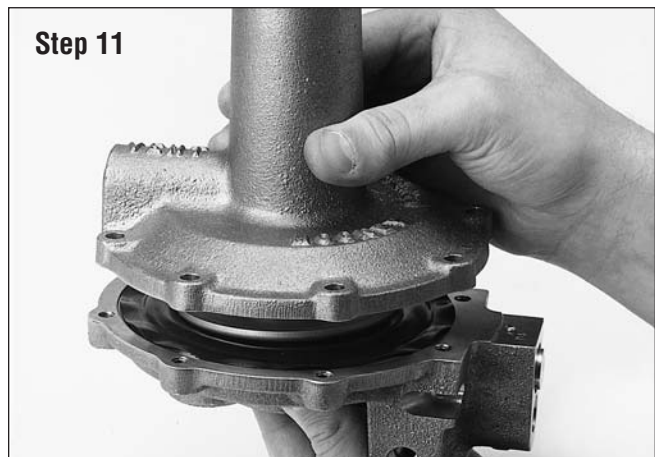
Figure 33 - Placing Spring Housing onto Pilot Body.
