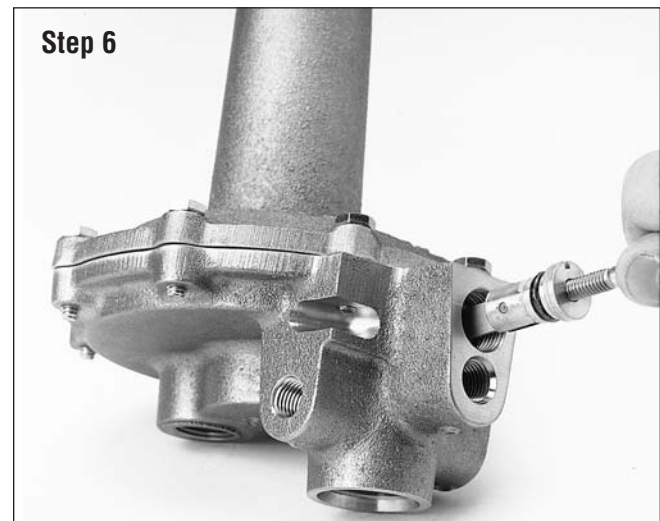
Figure 21. Pull the Pivot & Lever Assembly out of the Pilot Body.
