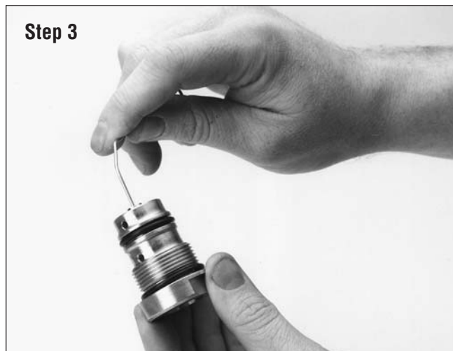
Figure 18 - The orifice can be pushed out of the Body Insert (Cartridge) using a paper clip.
