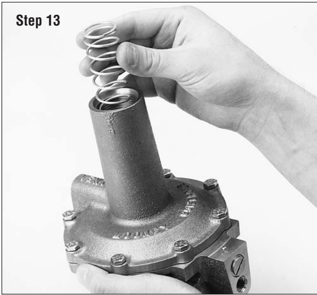
Figure 34 - Installing the Spring into the Spring Case.
